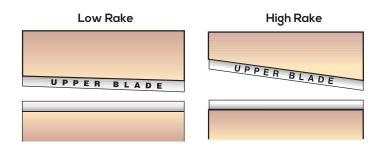
Variable rake is typically used for slitting purposes.
