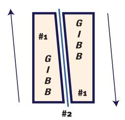
On each end of the shear ram is our EXTREMELY HEAVY-DUTY Gibbing system. This positive mechanical system provides a smooth, uniform gap adjustment via precision machined tapered gibbs. Each gibb plate (#1) slides opposite of each other on oil impregnated nylon call Nylatron (#2). These gibbs also control the front to back and left to right forces of the ram travel delivering the most precision cut available on any shear.
