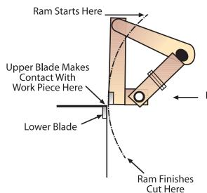
• The swing of the upper blade causes the angle or relationship of the top blade to the work piece to change throughout the stroke.
