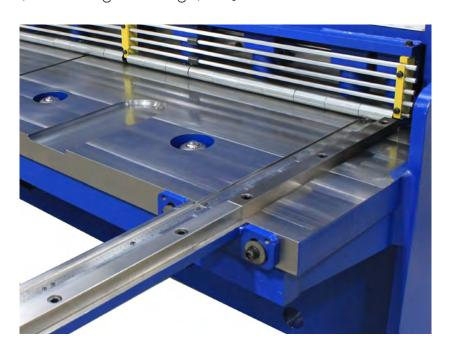
All 1/2" and 14" and longer shears are equipped with heavy duty ball transfers mounted in the table.
